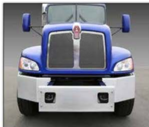
Kenworth's T470 grille is made of stamped stainless steel -- not plastic or pot metal. It's mounted to the radiator allowing the hood to swing clear of front mounted equipment. The bumper is constructed of three pieces for fast, economical installation of winches, PTOs and other front-end equipment.
